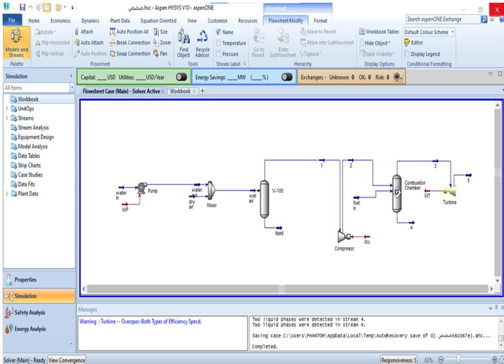
Figure 5 : Schematic diagram of the simulated turbine model without the fogging cooling system in Aspen Hysys
