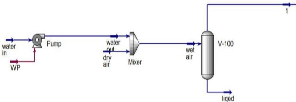
Figure 7: Fogging cooling Unit in Aspen Hysys
